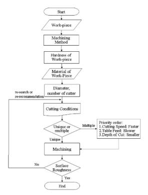
Fig. 2. Flow diagram of optimal cutting conditions for ballend milling.
