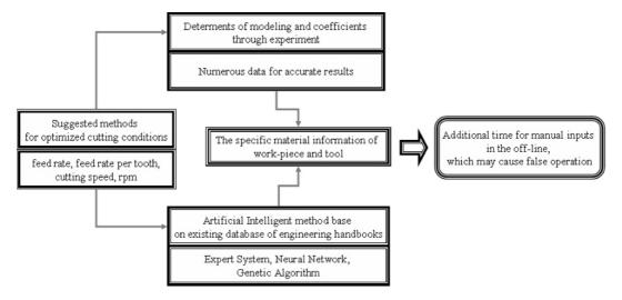
Fig. 1. Suggestion methods for optimized cutting conditions.
