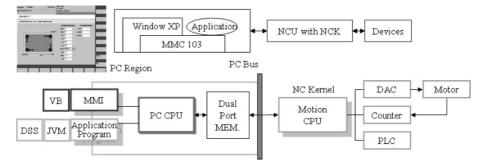
Fig. 3. Structure of open CNC controller.
