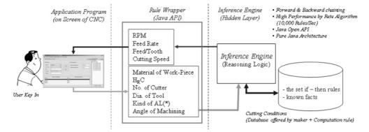
Fig. 5. Cutting condition recommendation system using rule-based knowledge Base.
